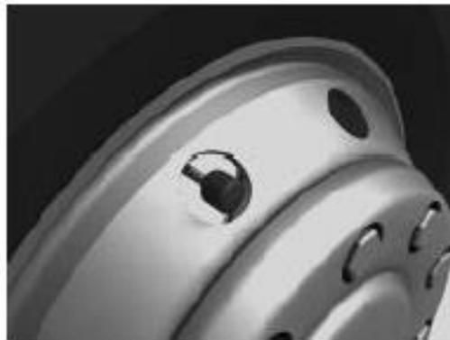
Figure 4 position of tyre sensor
