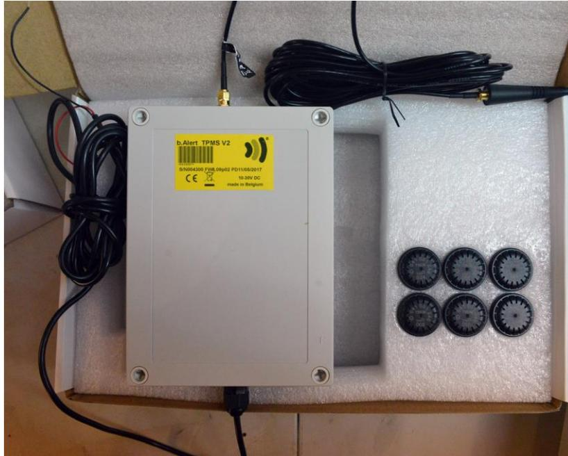
Figure 1 TPMS unit with sensors
